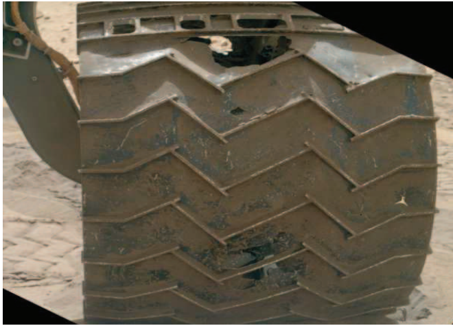
Fig 13. The perforation in wheels of Curiosity rover[22]
